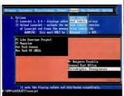
When Laserlet Setup Utility's menus refer to labels, the program means envelopes. This screen pops up when you want to edit an envelope, and the program keeps the same envelope in memory for future use. You can also save the return address or a whole envelope to a file.
